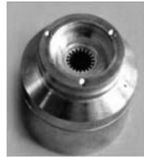
Fig. 27. Anakonda anode block with an insert of molybdenum.
