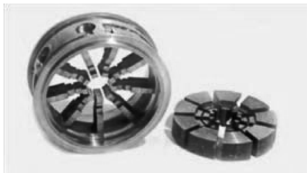
Fig. 24. Salyut amplatron anode block. Lamellae: a width of 4 mm and a height of 12 mm. D = 62 mm and d = 14 mm. The accuracy of manufacturing the components is 0.01 mm. The wastes are shown on the right-hand side.
