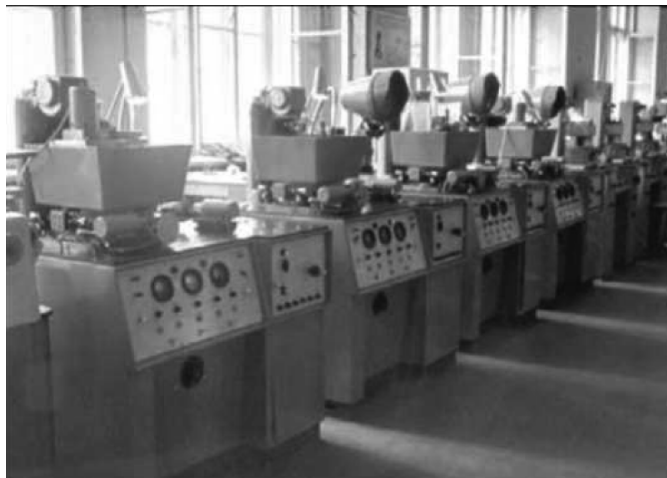
Fig. 22. Group of A207.33 installations with an embedded thyatron pulse generator and replaceable facilities for producing anode blocks, cathodes, and other components of electronic devices.
