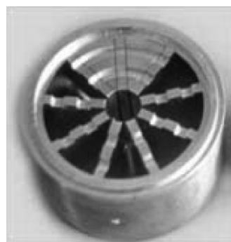
Fig. 25. Amplatron anode block: a height of 50 mm, D = 62 mm, and d = 14 mm. The lamellae are 4 mm. Seven resonators are cut.
