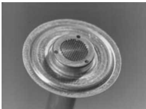
Fig. 7. Grid with a diameter of 7 mm having 152 square meshes with a size of 0.45 \times 0.45 mm and connecting strips between them of \leq 30 \mu\text{m} prepared in the diaphragm of a klystron.
