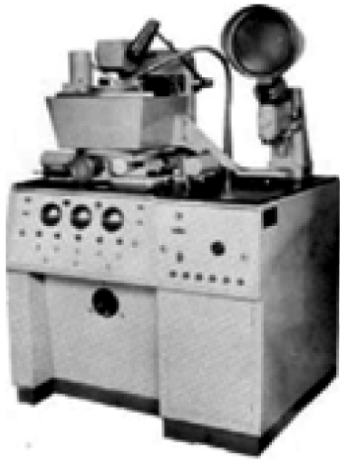
Fig. 17. A207.33 installation with an embedded thyratron pulse generator.
