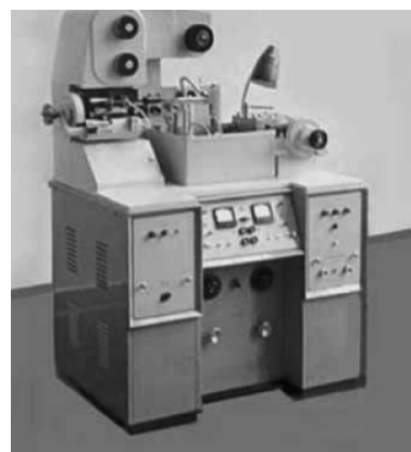
Fig. 16. A207.27 electrospark machine for producing M-type device anode blocks using two wires with an embedded thyatron pulse generator.
