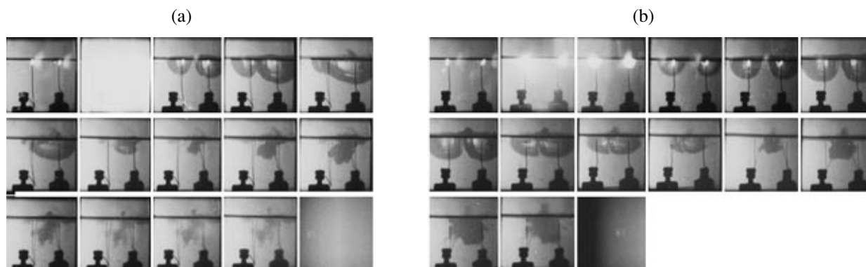
Fig. 5. Elements that control the cavitation region for parallel electrical discharges: (a) when initiation of one of the discharges is substantially delayed ( \Delta t = 8 \mu\text{s} ); (b) strictly synchronous discharges ( \Delta t = 0 ), for working voltage U_1 = 17.8 \text{ KV} (frames 11–14).
